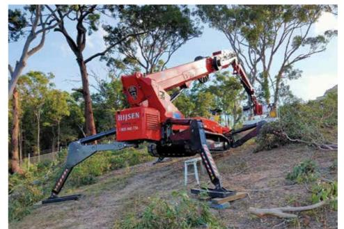
with the unique telescopic fly jib and platform rotation, the 43T Spider Lift will also allow operators to manoeuvre the basket into the work zone with fine precision. And once the job is complete, hold in the 'Auto-Stow' button and the machine fully stows the booms for you.
